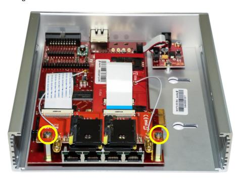
After the box has been opened the GSM\_Extension Kit has to be lifted up in order to reach LineInterface 0 (LIO).
