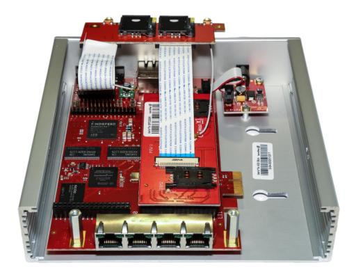
Now the LineInterface 0 (LIO) can easily be reached so you can place your chosen module which the box has to be upgraded with.
