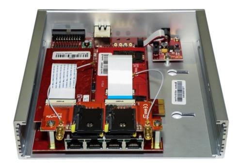
In case of upgrading the GSM Gateway with an additional 2GSM module it has to be connected with the GSM\_Extension Kit. Use the pre-attached cables on the GSM\_Extension Kit.
