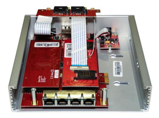
After the Gateway has been upgraded attach the GSM\_Extension Kit back to its previous position.
