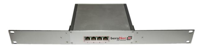
In order to attach the 19" brackets to the gateway use the 3 mounting threads on the sides of the gateway.
