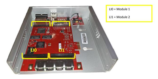
First you should place the module softly on one of the beroNet Gateway module slots. There is only one possible direction since one side of the module has a male and the other side has a female connector.
