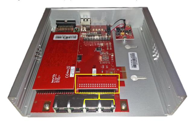
Since a beroNet Gateway has only 4 RJ45 ports but can be equipped with 2 modules in total containing up to 8 ports, it is necessary to break out the 4 additional ports. Therefore you need the BNTAdapters.
