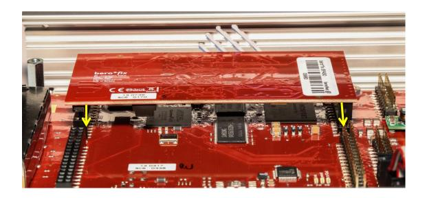
In case of a single 4 port module it is recommended to use the included BFBridge. Placing the BFBridge on the LineInterface 1 (LI1) will unlock the two additional RJ45 ports.
